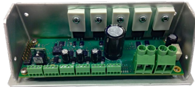
The SR-54 Programmable temperature controller deliver a complete thermal management solution when combined with a thermoelectric cooler assembly.
