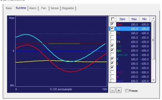
Runtime tab allows user to visually monitor operation parameters of controller. A live running time scale graph appears that allows user to view main power, thermistors, temperature set points, input current draw, input voltage to TEMs, input power to fans and PID parameters.
