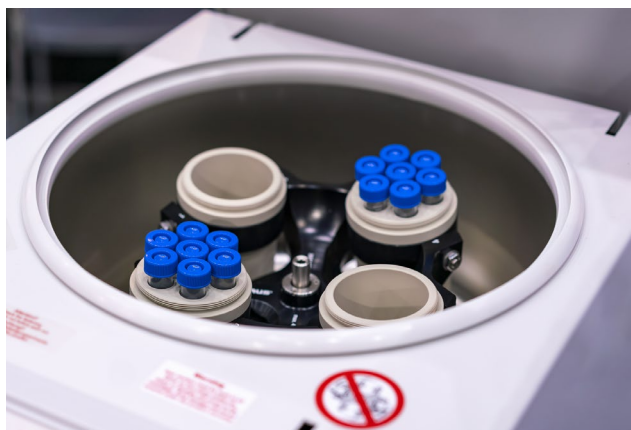
Centrifuges use centrifugal force to separate mixtures.
