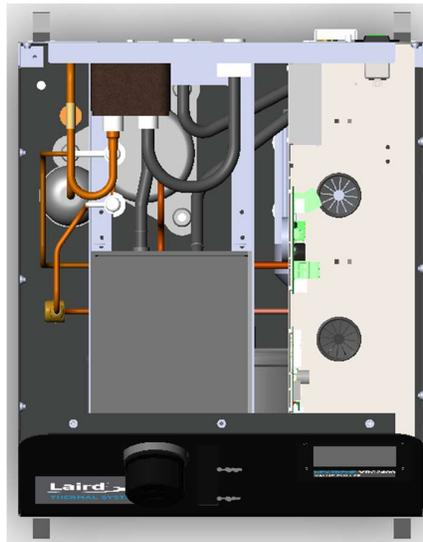
Figure 3 Top View of VRC1200 and VRC2400
