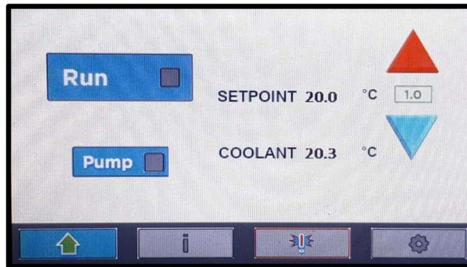
Figure 24 Home screen with an active alarm
