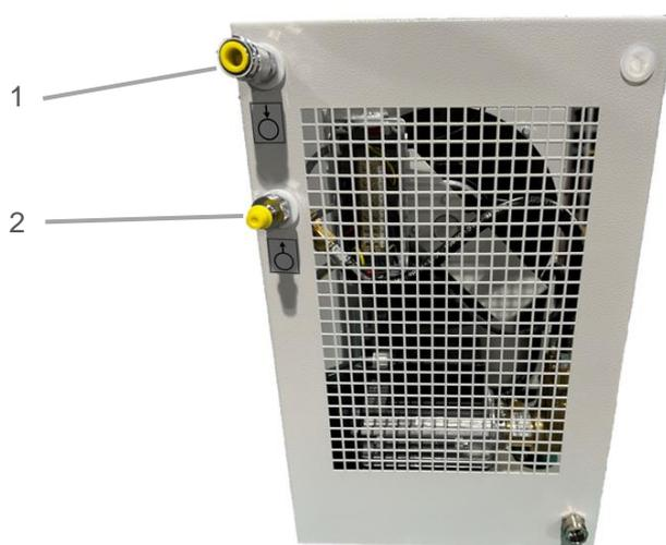
*Fig. 12: Inlet and Outlet Ports for Draining*
