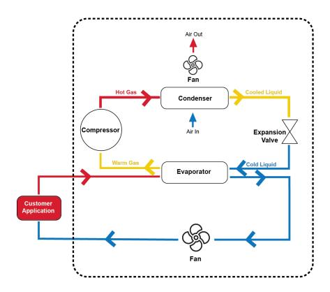
A conventional compressor-based refrigeration system contains four fundamental parts: the evaporator, compressor, condenser, and expansion device. The evaporator (cold section) is a heat exchanger where the refrigerant interfaces with the process fluid (air or liquid coolant in the
