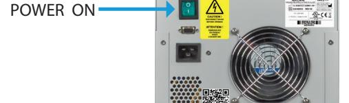
**Turn on the power switch on the back of the unit.**
