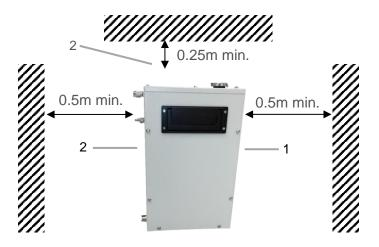
Fig. 6: Minimum clearance for air entrance and air exit
